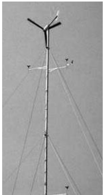
A temporary tower, equipped with wind-measurement technology, takes readings at a potential wind-turbine site.
